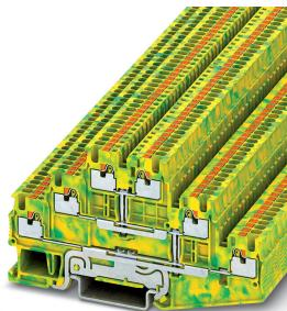
Ground modular terminal block, nom. voltage: 500 V, nominal current: 15 A, connection method: Push-in connection, 1 level, Rated cross section: 1.5 mm<sup>2</sup>, cross section: 0.14 mm<sup>2</sup> - 1.5 mm<sup>2</sup>, mounting type: NS 35/7,5, NS 35/15, color: green-yellow
